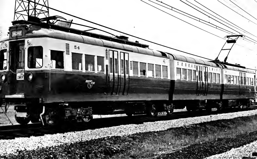
One of the four 96-seat articulated cars added to bolster passenger capacity. Like the small standard cars, these are all electric. The main service brake is dynamic, with spring applied, solenoid released, drum parking brakes. Magnetic track brakes and track sanders are also provided for additional control in event of marginal rail surface conditions.
